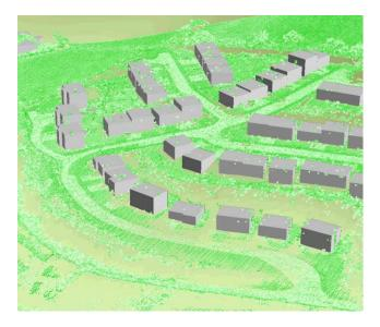
Figure 2: Sample Point Cloud from Aerial LiDAR Survey
